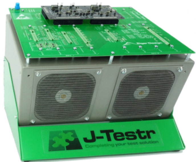
Picture: J-Testr fitted with demonstration interposer
